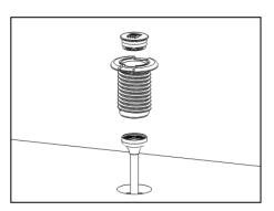
4. Remove the remaining installed light assembly from the underside of the hole.
