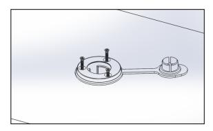
9. Use a screwdriver or drill to drive the three screws into the adapter ring from the top side.
